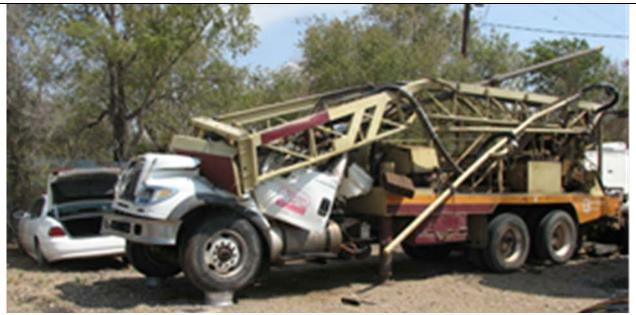
Figure 3. Example cab deformation with tower in stowed position
