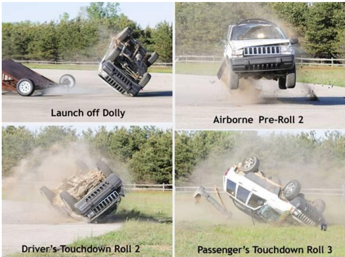
Figure 10. HALO™ Prototype 4 during a FMVSS 208 dolly rollover test
