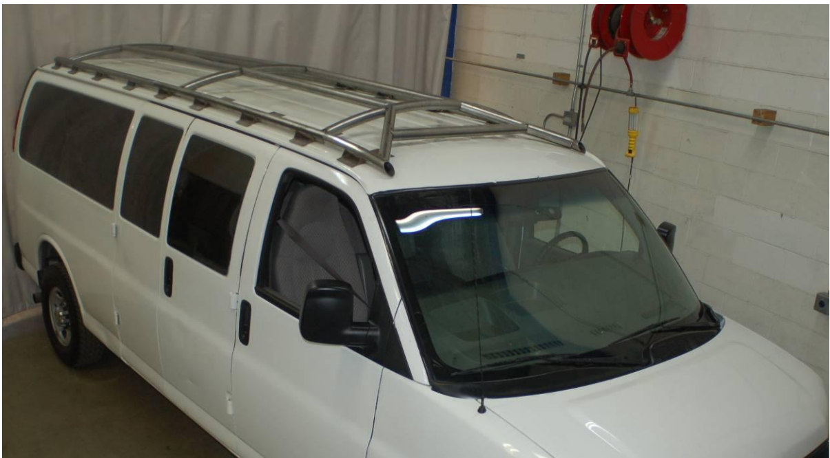
Figure 18. 12 to 15 Passenger van with HALO™ rollover load distribution device.
