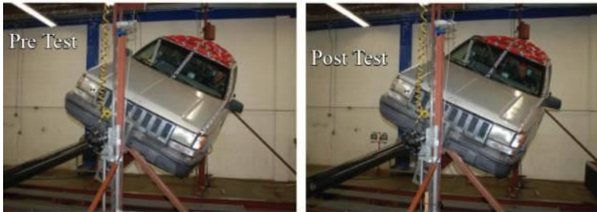
Figure 6. HALO™ Prototype 2; No noticeable deformation to the roof structure
