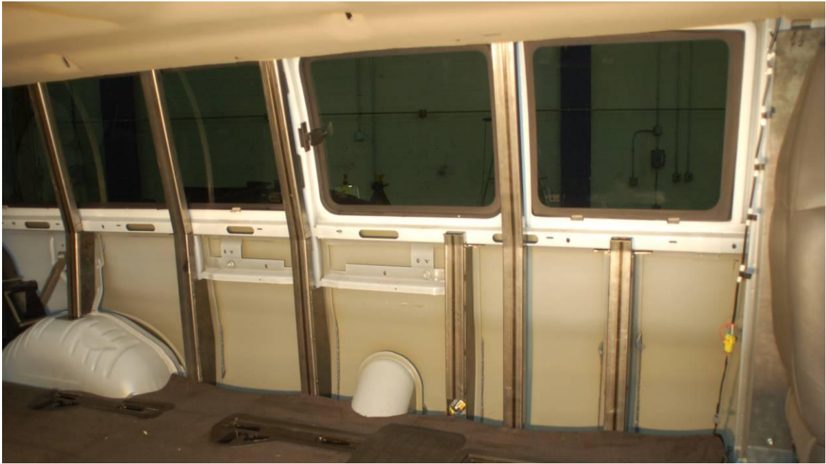
Figure 17. Passenger van internal retrofit strengthening system
