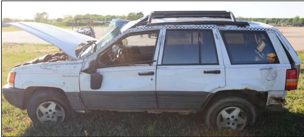
Figure 11. Prototype 4 HALO™ after a 3 roll dolly rollover test
