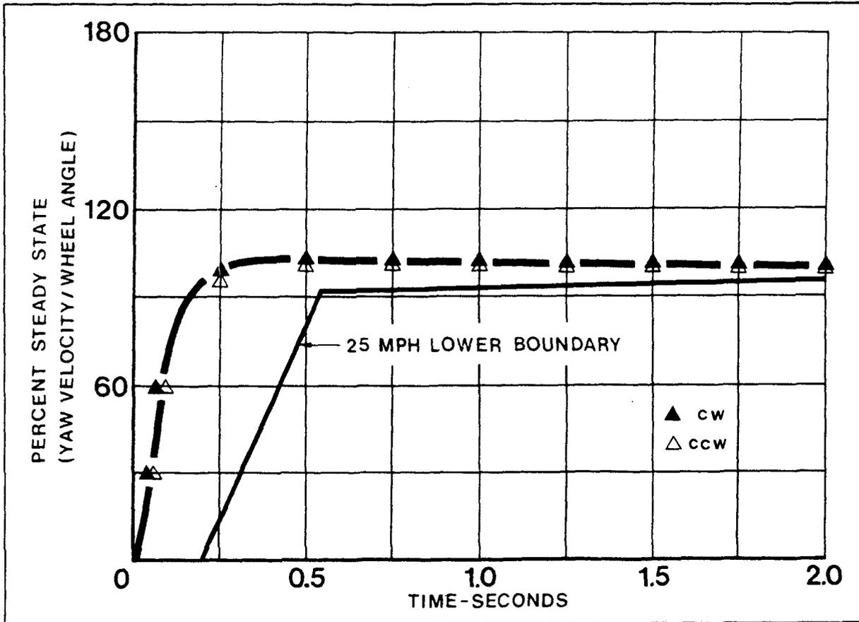
Figure 11. Minicars RSV transient yaw response at 25 mph.
