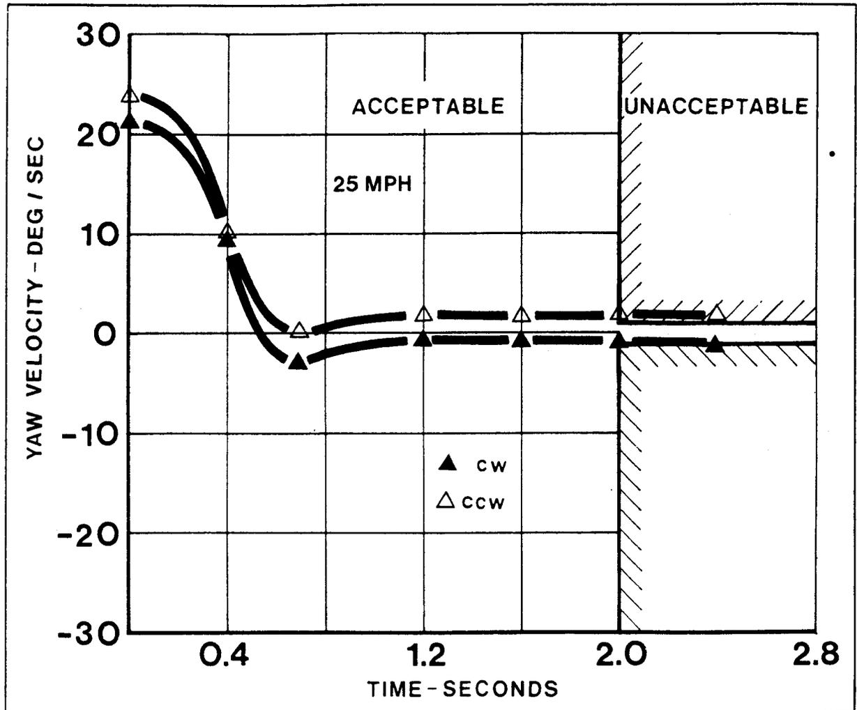
Figure 14. Minicars RSV returnability performance yaw rates at 25 mph.
