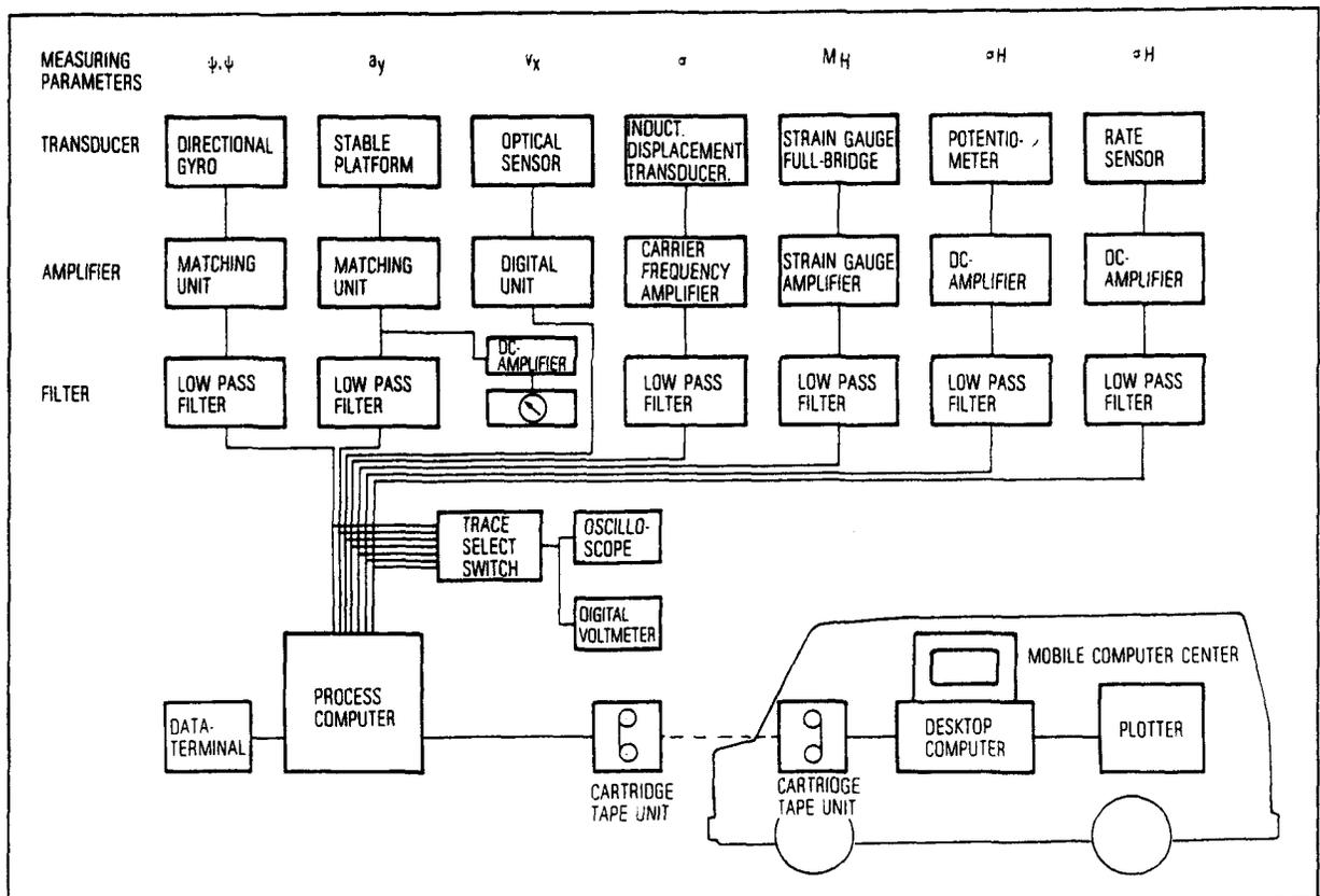
Figure 4. Minicars RSV measuring arrangement.
