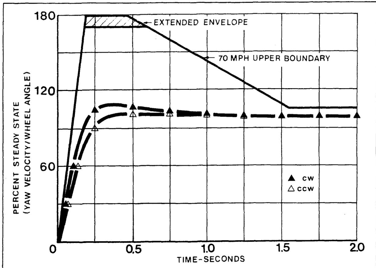
Figure 12. Minicars RSV transient yaw response at 70 mph.
