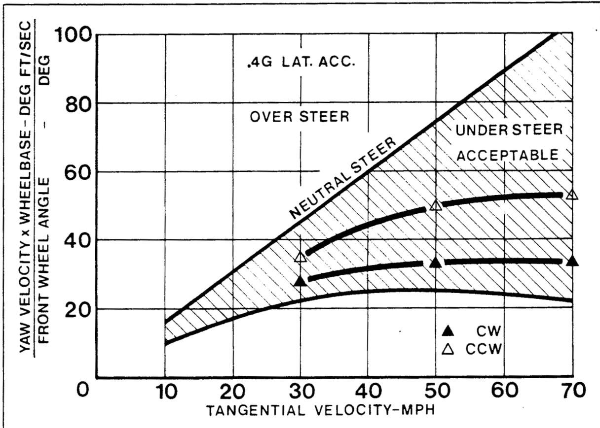
Figure 10. Minicars RSV steady-state yaw response.
