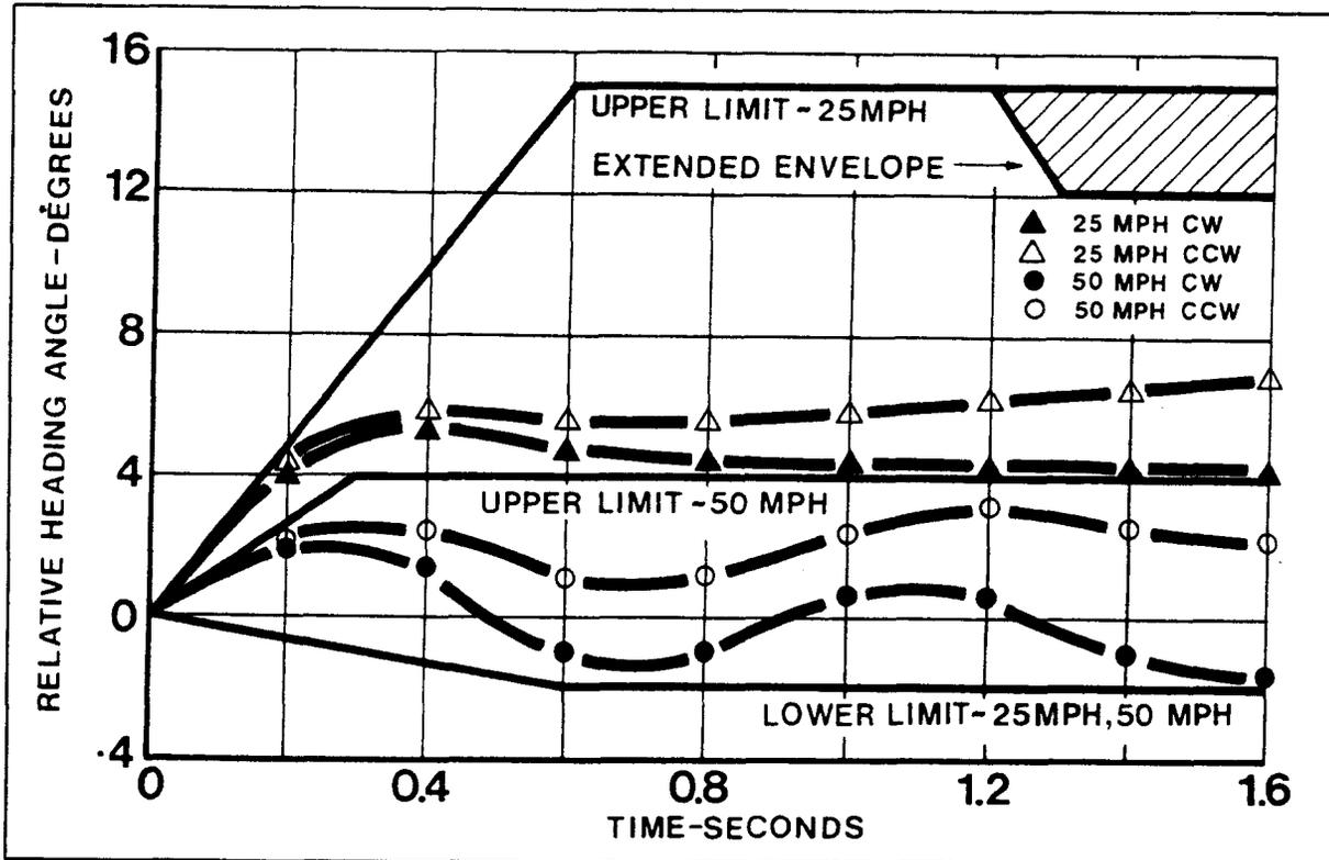
Figure 13. Minicars RSV Steering returnability free control heading.
