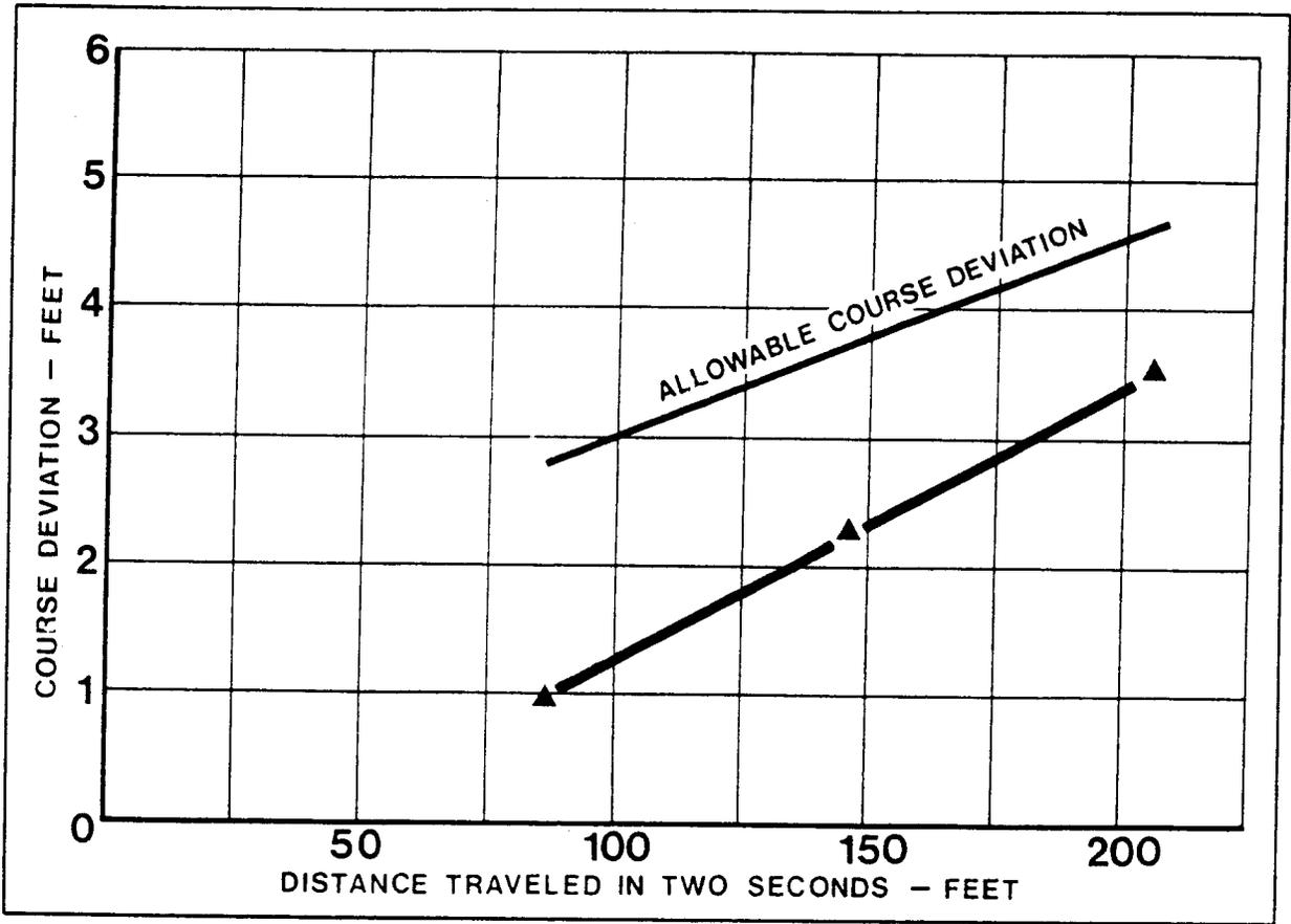
Figure 17. Minicars RSV crosswind sensitivity allowable course deviation by crosswind.
