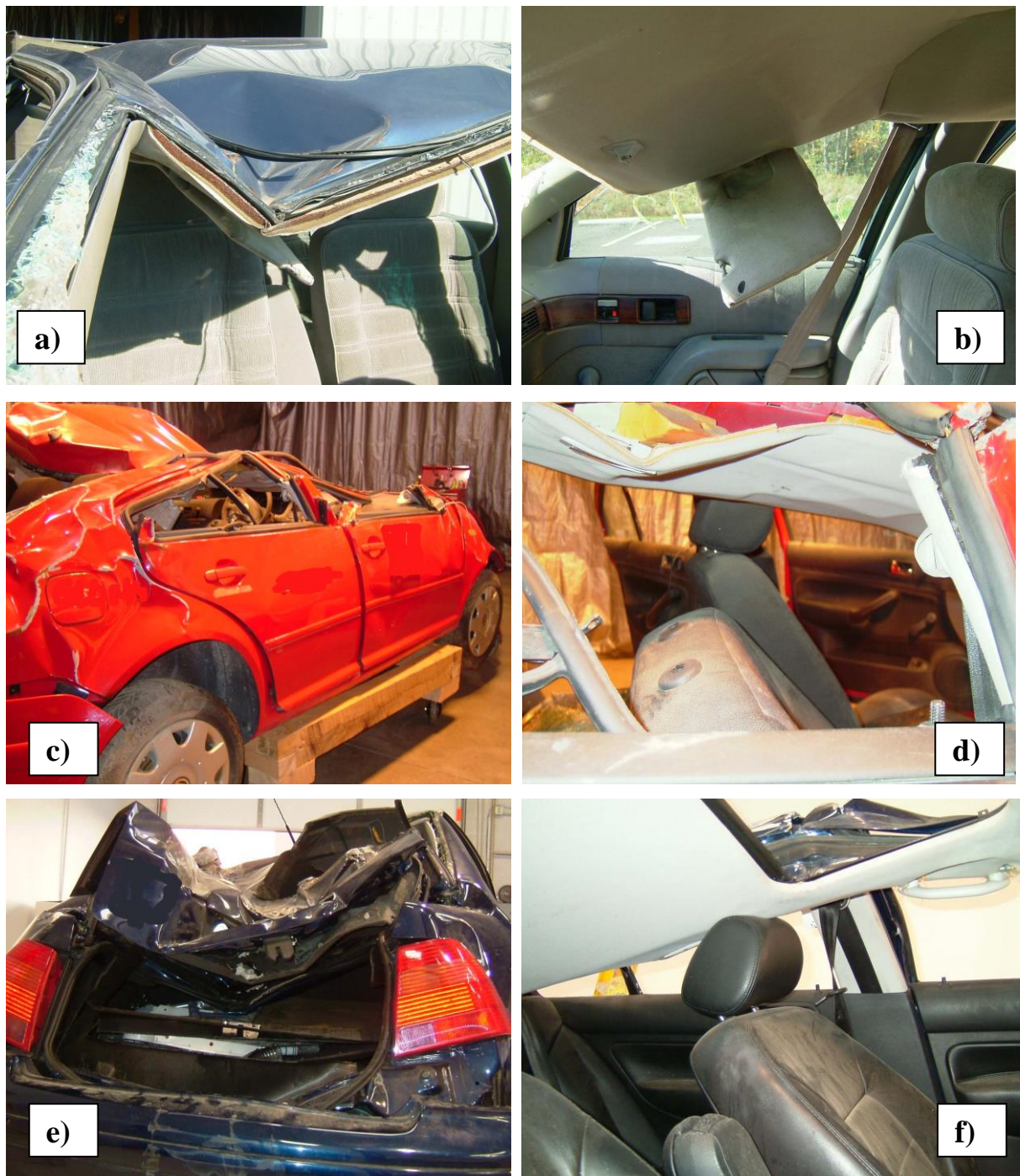
Figure 4. External view of roof deformation and internal view of roof intrusion
