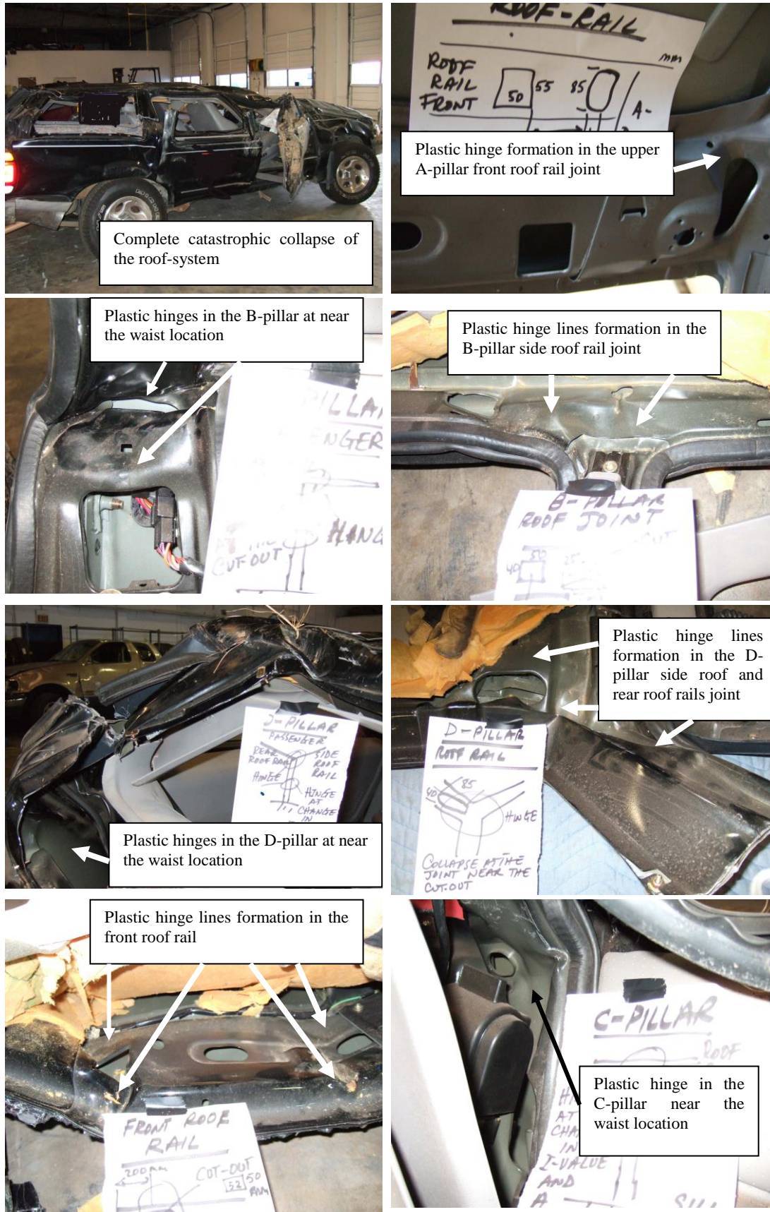
Figure 6. Collapse mechanisms occurring at cut-outs locations in a typical SUV under rollover
