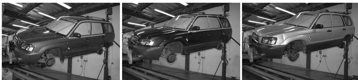
Figure 1. Photographs of the Three Subaru Foresters before the First Roll on the JRS.
