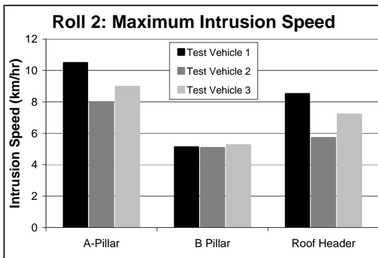
Figure 13. Maximum Roof Intrusion Speed During the Second Roll.
