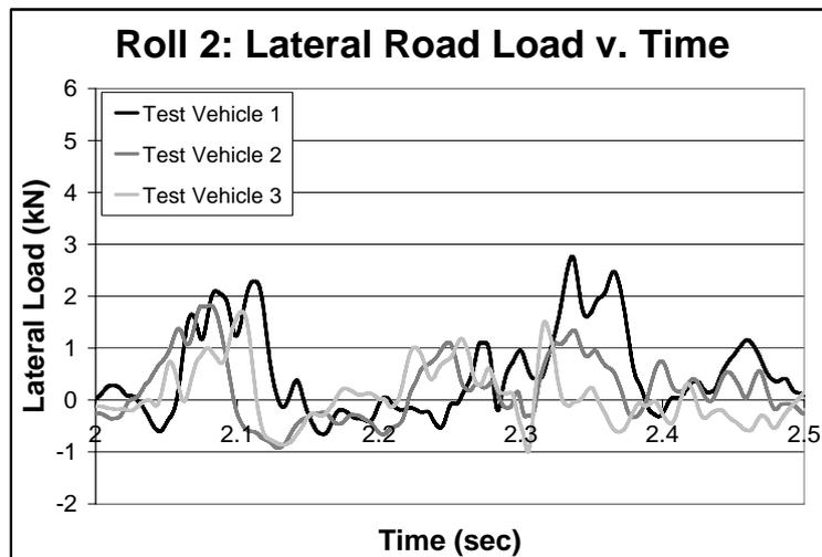
Figure 10. Lateral Road Loads for Roll 2.
