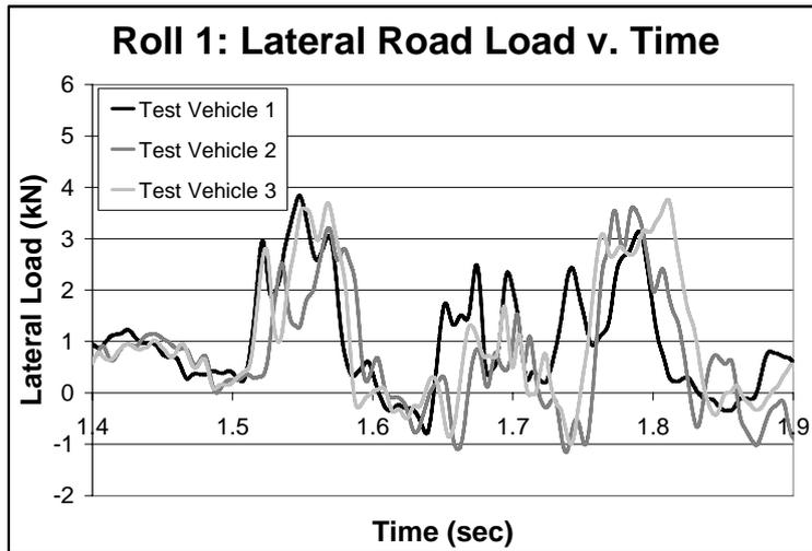
Figure 4. Lateral Road Loads for Roll 1.
