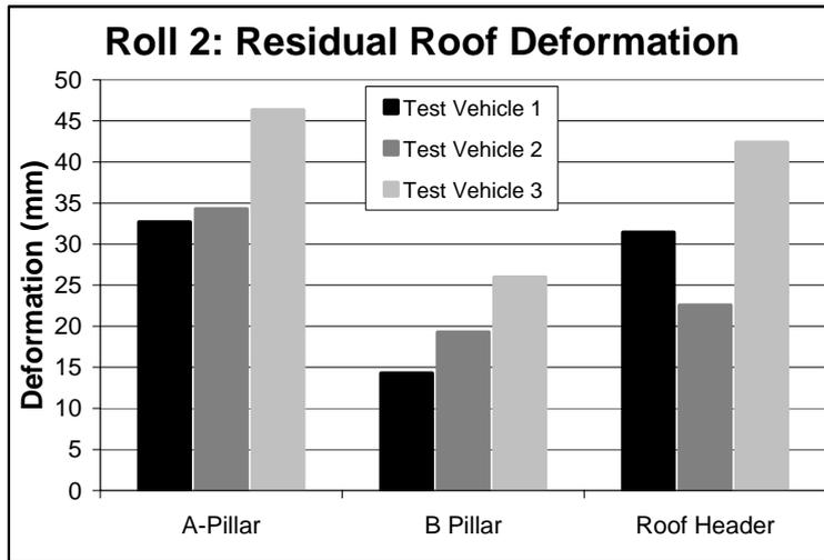
Figure 12. Residual Roof Crush Following the Second Roll.
