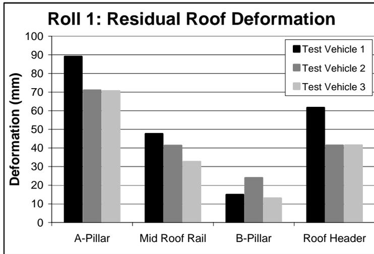
Figure 6. Residual Roof Crush Following the First Roll.
