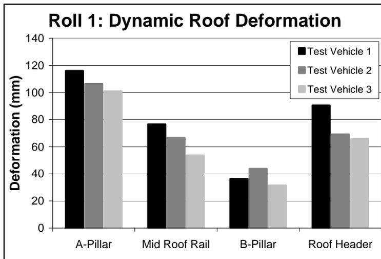
Figure 5. Maximum Roof Crush During the First Roll.
