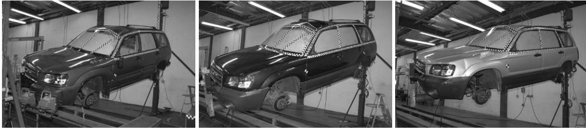
Figure 2. Photographs of the Three Subaru Foresters Following the First Test on the JRS.
