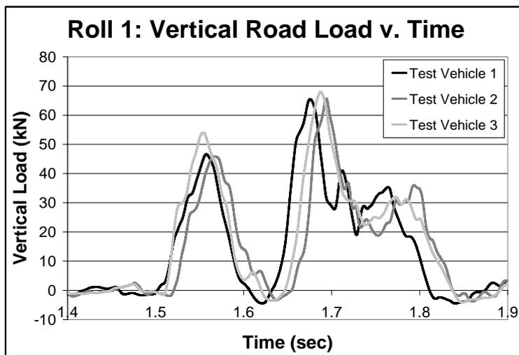
Figure 3. Vertical Road Loads for Roll 1.
