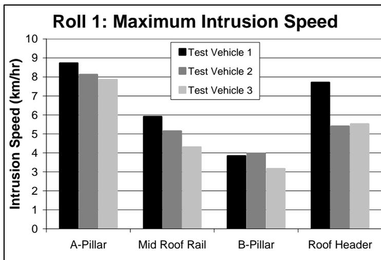
Figure 7. Maximum Roof Intrusion Speed During the First Roll.
