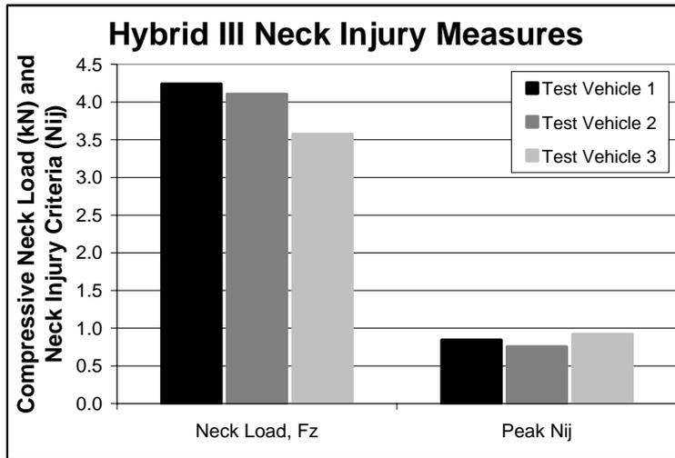
Figure 14. Hybrid III Neck Injury Measures: Compressive Neck Load and Neck Injury Criteria.
