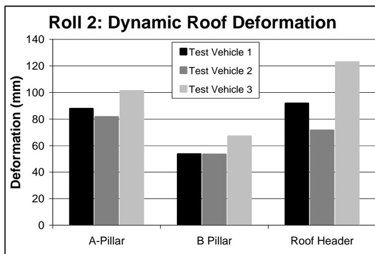
Figure 11. Maximum Roof Crush During the Second Roll.
