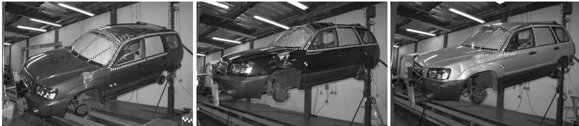
Figure 8. Photographs of the Three Subaru Foresters Following the Second Roll on the JRS.
