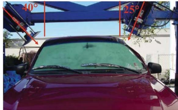
Figure 5. Vehicle in M216 test fixture.
