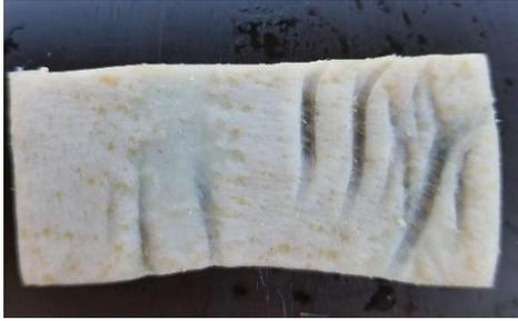
Figure 8. Damage patterns from plastic edge
