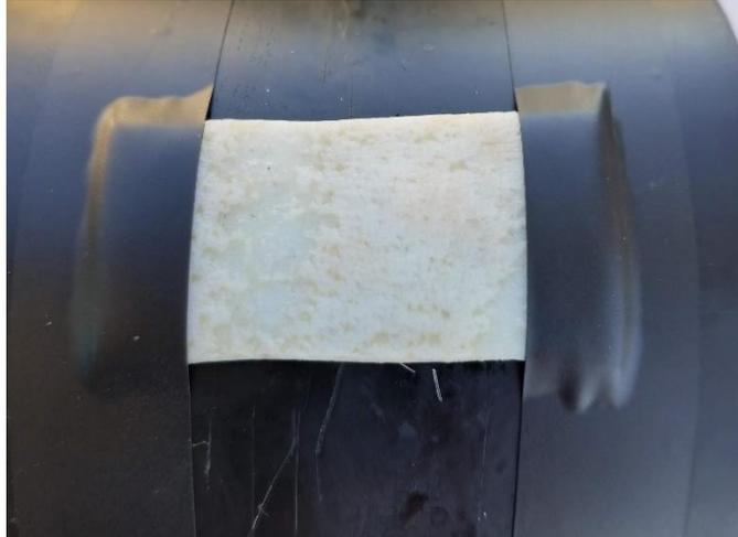
Figure 3. Porcine skin specimen constrained to backing surface
