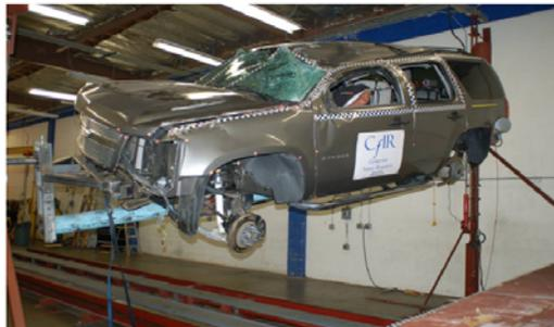
Figure 4: Vehicle Post Roll 2
