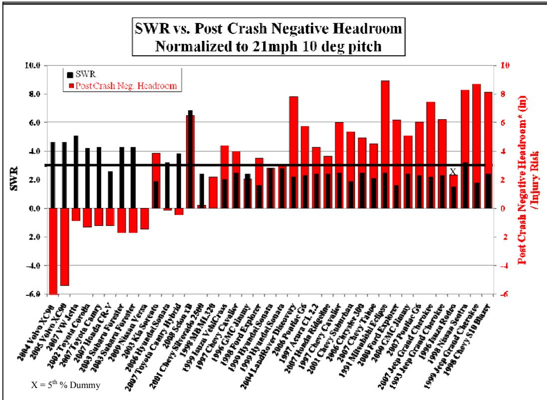
Figure 5. The relationship between post crash negative headroom and SWR
