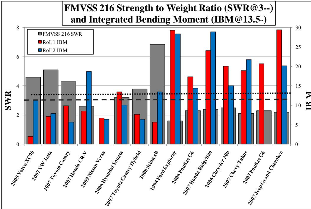
Figure 6. The relationship between the Integrated Bending Moment (IBM) and SWR
