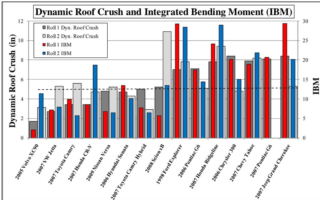
Figure 7. Dynamic Roof Crush and Integrated Bending Moment (IBM@13.5--)
