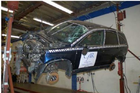
Figure 2: Vehicle Post Roll 1
