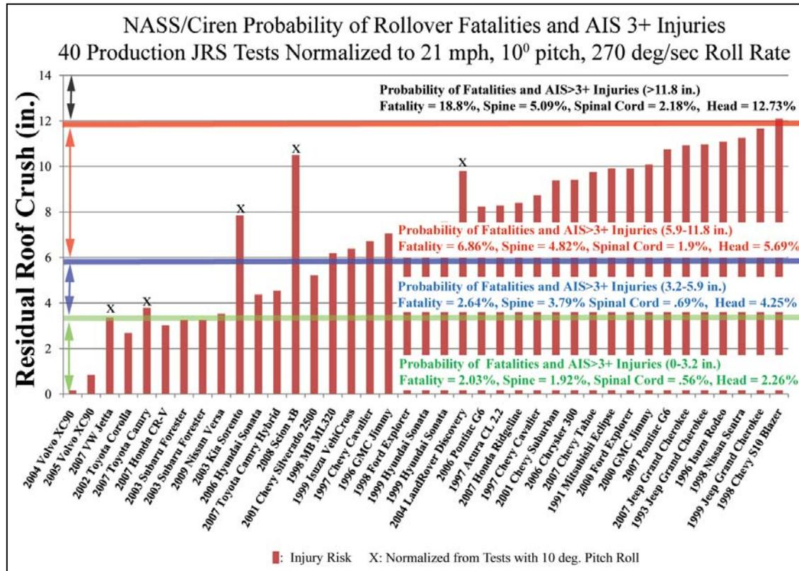
Figure 4. Residual crush of 40 normalized JRS tested production vehicles with NASS/Ciren probability of fatality and AIS ≥ 3 injury.
