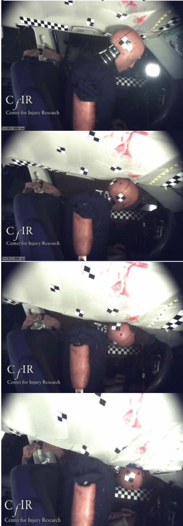
Figure 12. Dummy in roll 2 of the Scion xB test
