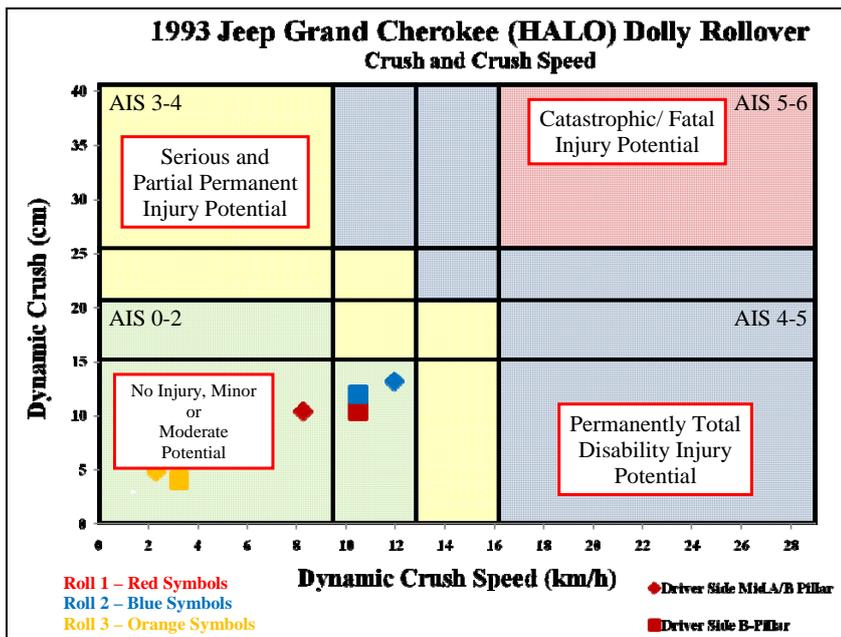
Figure 27. RDMD Dolly Rollover Results with ¾ b-pillar reinforcements on AIS injury chart.
