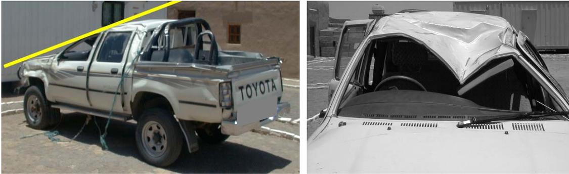
**Figure 2. Vehicle reinforced with internal roll bar at B-pillar and external roll bar behind C-pillar. Note buckle of front windshield header rail intruding into occupant compartment.**
