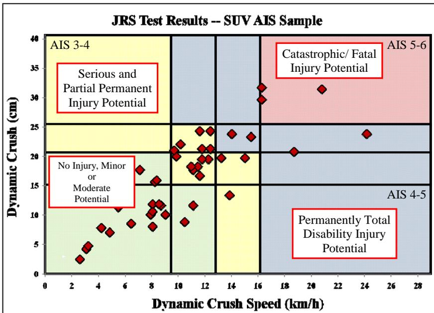
Figure 22. Range of SUV vehicle test results on the JRS.
