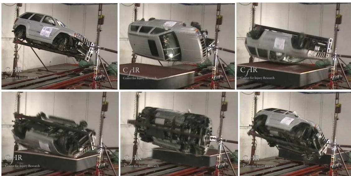
Figure 10. Still frames of a JRS test. Note: frame 3 near side strikes floor; Frame 4 far side strikes floor.
