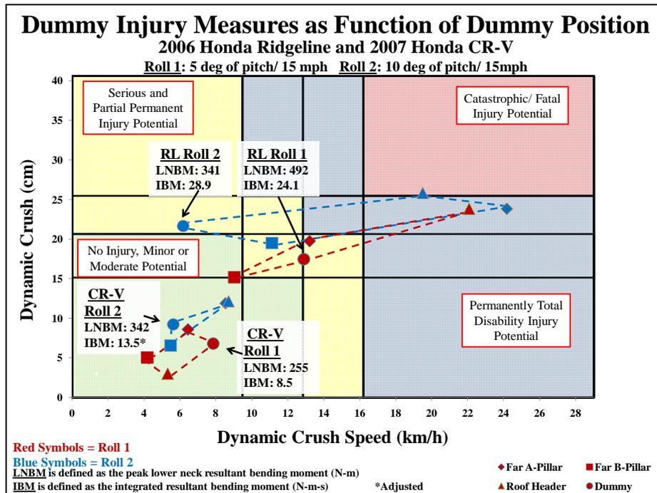
Figure 32. Potential injury is a function of occupant position relative to the roof components.
