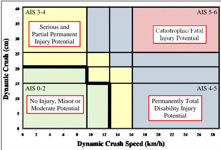
Figure 21. AIS Injury Scale for Motor Vehicle Accidents by Crush and Crush Speed
