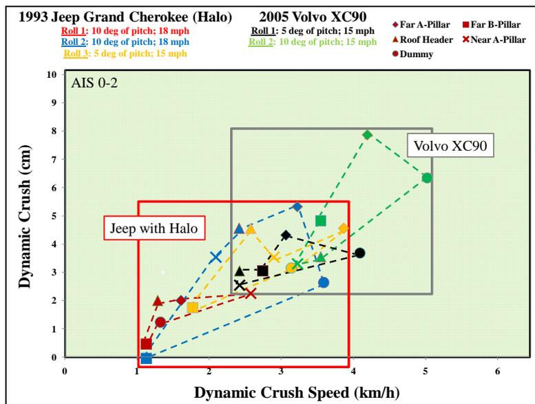
Figure 29. Blow up of AIS 0-2 range for Jeep with RDMD HALO compared to Volvo XC90
