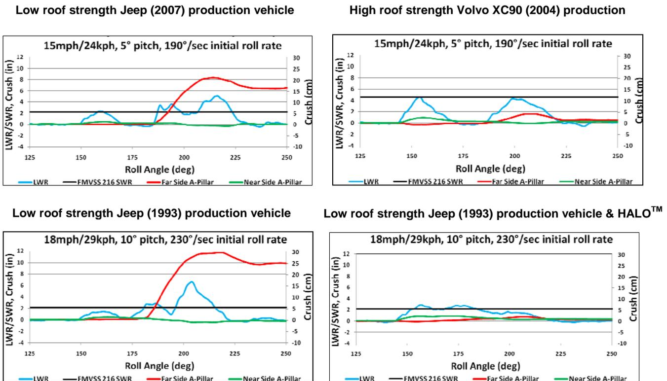
Figure 17. Loads measured in moving floor for: low roof strength (1993 & 2007) production vehicles; high roof strength vehicle; and low roof strength (1993) vehicle with RDMD.
