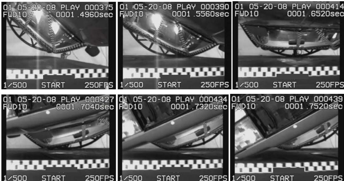
Figure 16. ATD interaction with (1993) low roof strength vehicle's (SWR 2.3) roof and floor during near side and far side touchdown. ATD's head is circled.
