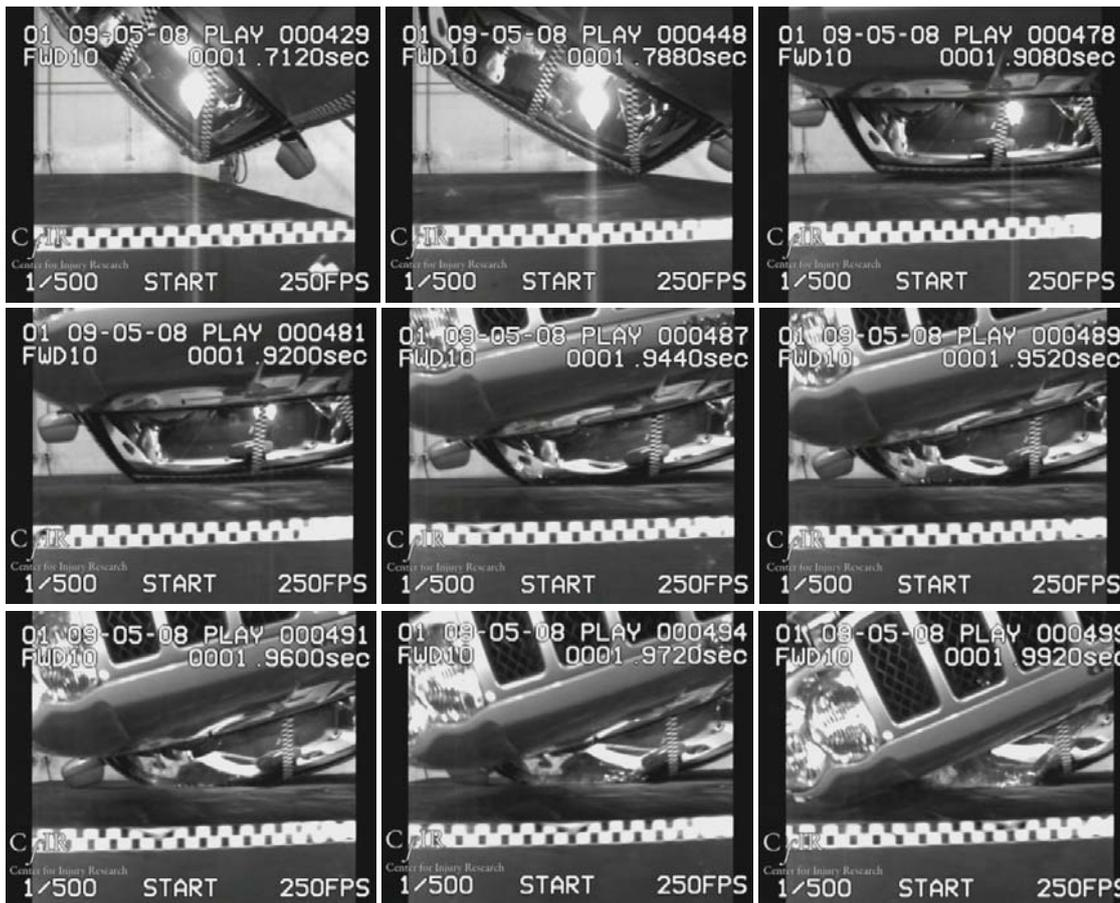
Figure 13. ATD interaction with low roof strength vehicle's (SWR 2.2) roof and floor during near side and far side touches down.
