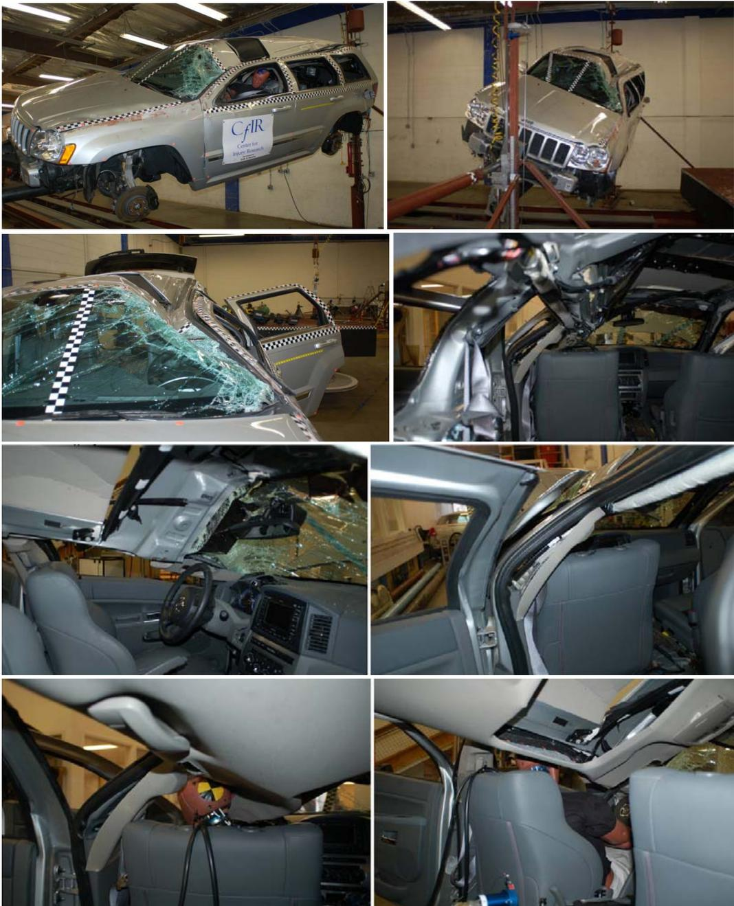
Figure 11. Deformed roof structure of low roof strength (SWR = 2.2) vehicle after roll 2 JRS test.
