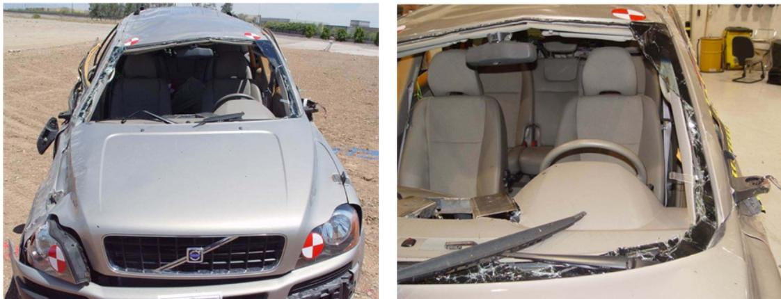
Figure 20. 2004 Volvo XC90 post test photos – 70 km/h (44 mph) Dolly Rollover Test
