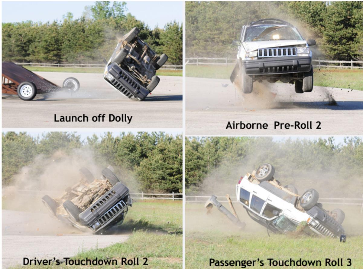
Figure 25. Sequence of photo's from 42 mph Dolly Rollover test of 1993 Jeep Grand Cherokee with RDMD HALO.
