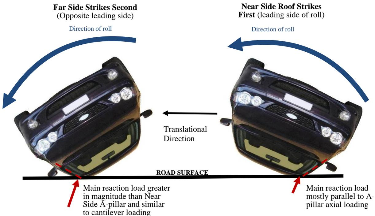
Figure 8. Loads applied to vehicle's roof during rollover.
