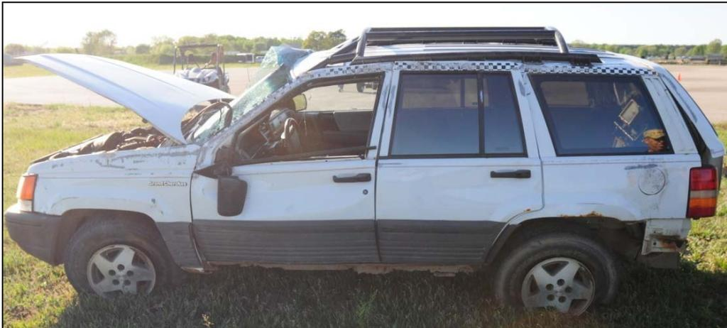
Figure 26. 1993 Jeep Grand Cherokee after 3 roll Dolly Rollover Test with RDMD attached.
