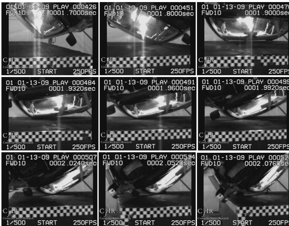
Figure 14. ATD interaction with high roof strength vehicle's (SWR 4.6) roof and floor during near side and far side touchdown.
