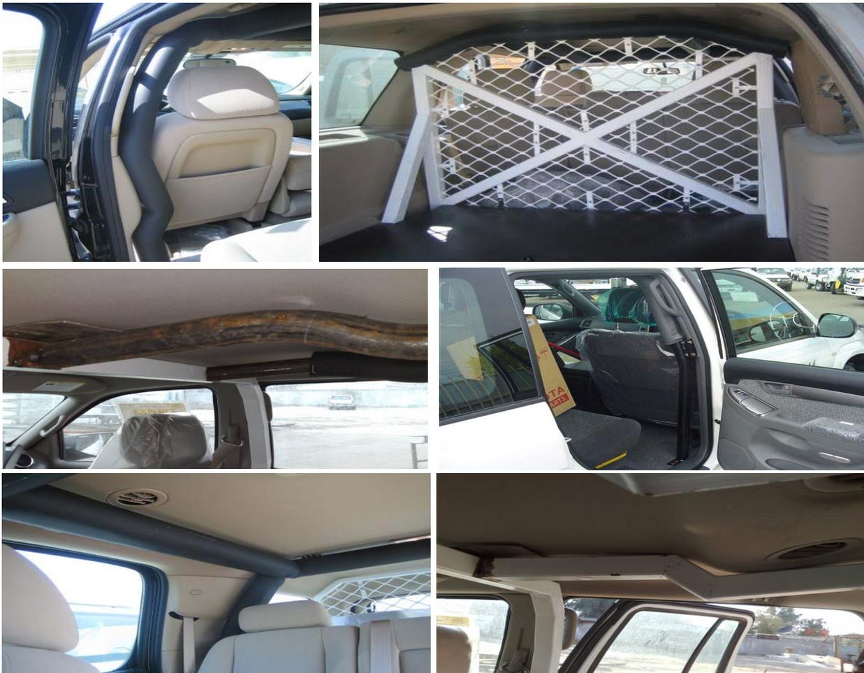
Figure 1. Examples of roof strengthening using internal rollover bars.
