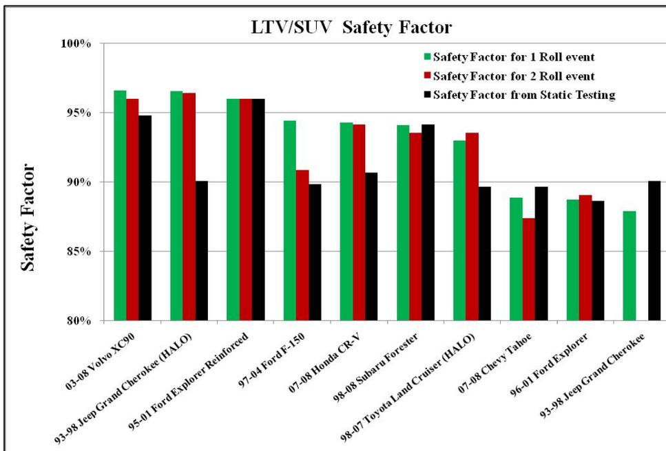
Figure 30. Tested production and modified SUV safety factor relationship for 10 vehicles
