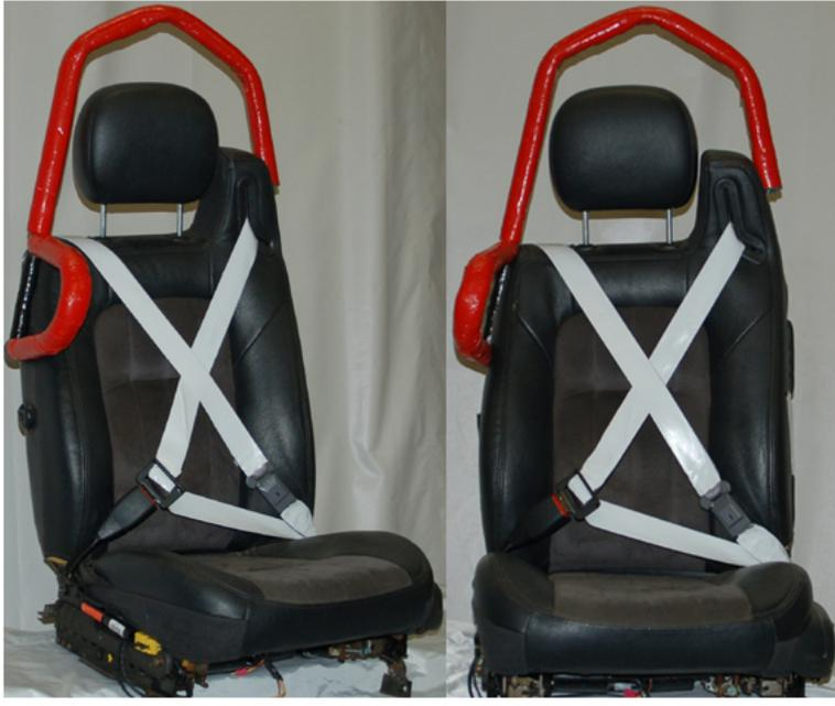
Figure 33. Prototype All-Belts-to-Seats Occupant Protection System.
