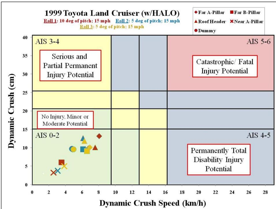
Figure 24. 1999 Toyota Land Cruiser Dynamic Test Results with RDMD attached.
