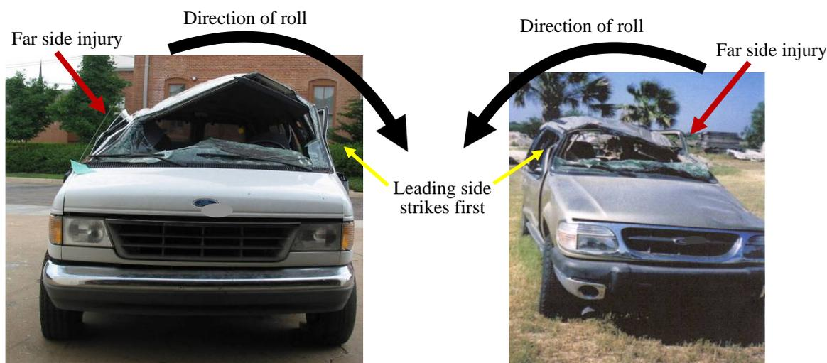
Figure 7. Two different vehicles where the injured were on the far side of the roll direction where the roof crushed.
