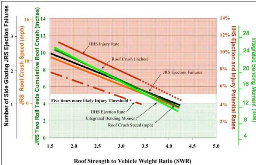
**Fig 2. Composite plot of injury measures showing rate reduction with increasing vehicle SWR.**
