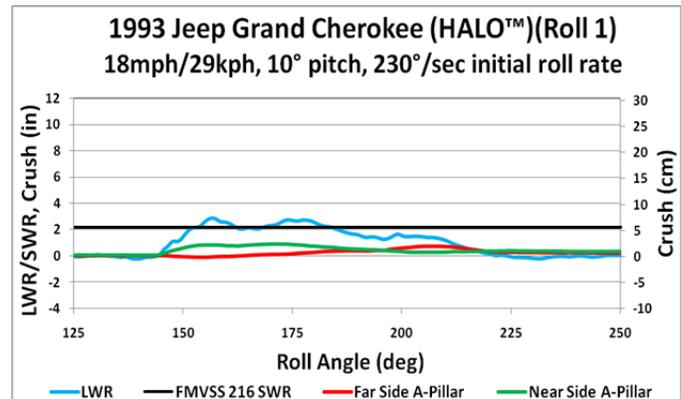
Fig 20. Road loads in blue and A-Pillars in red and green.
