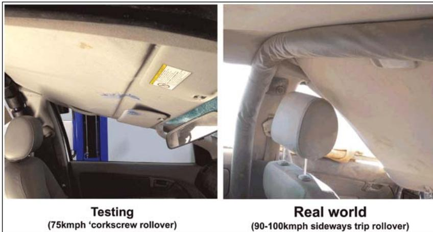
**Fig 11.** Comparison of the internal post crash photo of the tested ROPS Hilux and a real world rollover.
