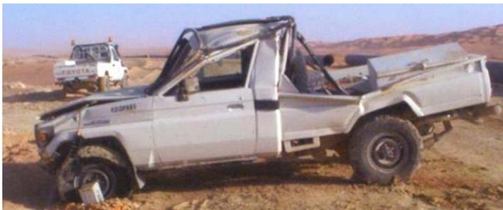
Fig 16. Real World rollover of vehicle with Safety Device ROPS.
