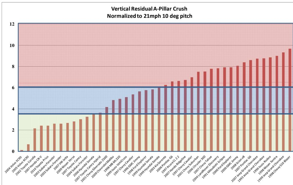
Fig 5. Residual crush normalized to 21 mph and 270° roll rate.
