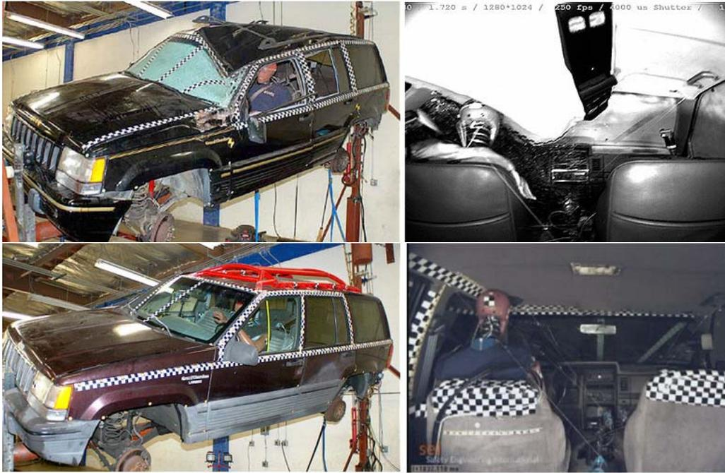
Fig 17. HALO JRS rollover testing, production vehicle on top and HALO equipped vehicle on bottom.
