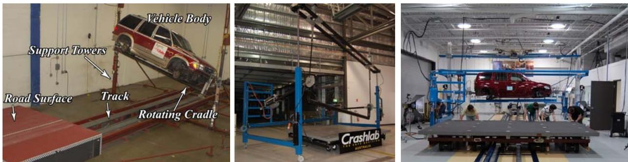
**Fig 13.** Lateral dynamic JRS rollover test devices in California, Australia and the Commonwealth of Virginia.
