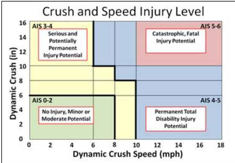
Fig 6. Consensus injury criteria map of dynamic crush and crush speed injury risk criteria.
