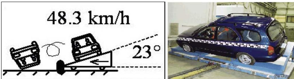
**Fig 12.** Lateral dolly rollover basic test configuration.
