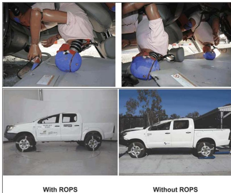
Fig 10. Ramp Rollover testing with and without an internal 4 posted ROPS device.
