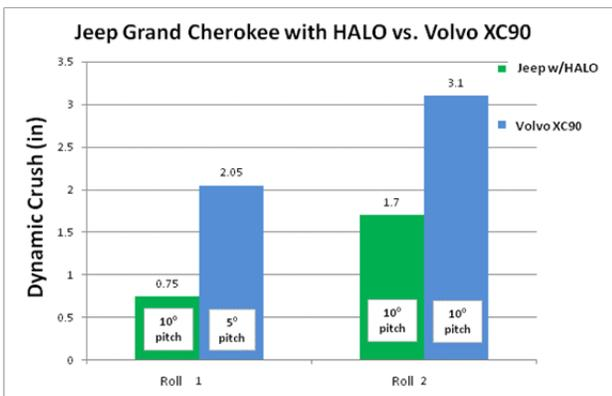
Fig 19. Jeep with HALO vs. Volvo XC90.
