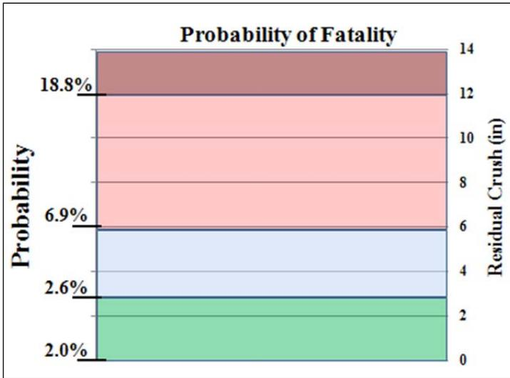
Fig 4. Fatal probability function vs. residual crush in inches.
