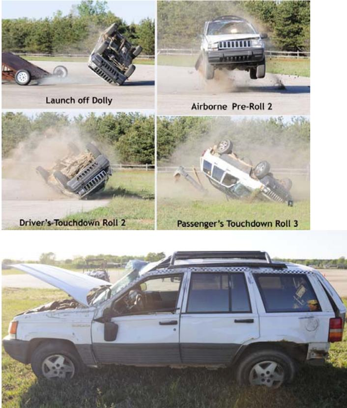
Fig 21. HALO ROPS dolly Rollover testing.
