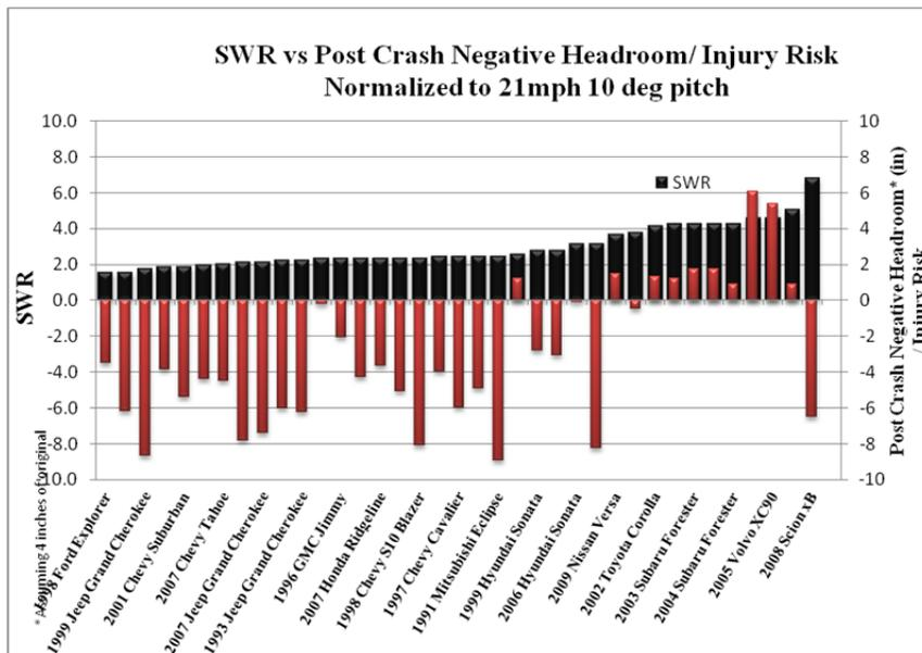
**Fig 3. Post-crash positive and negative headroom in order of ascending vehicle SWR.**
