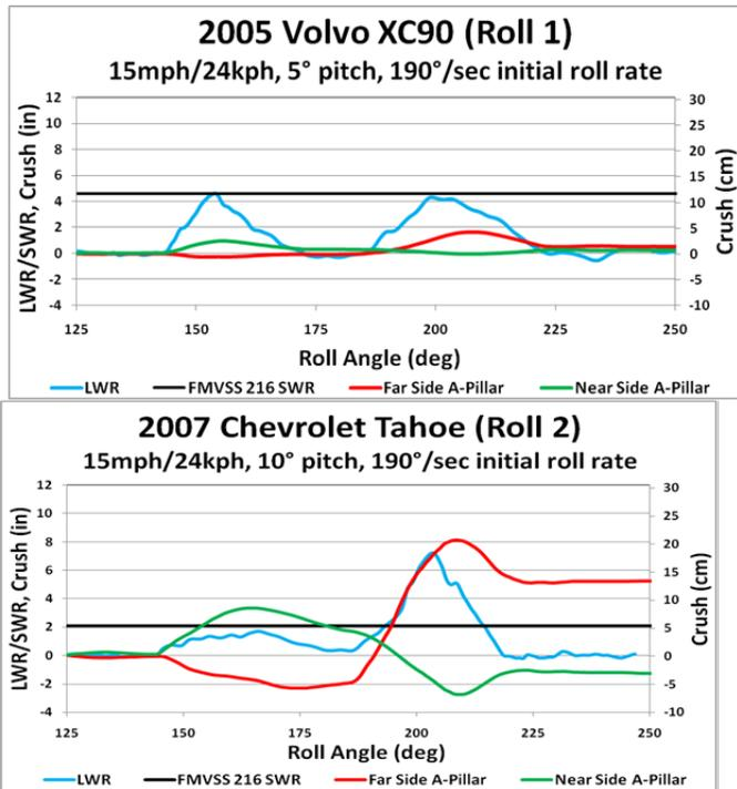
Fig 22. Comparison of Road Loads in JRS testing with a strong (Volvo XC90) and weak roof (Tahoe) vehicle.
