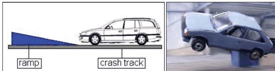
Fig 9. Ramp rollover basic test configuration.
