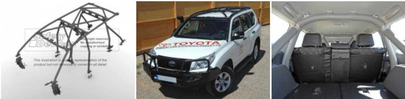
Fig 15. Safety Device's Roll Over Protection Rack.
