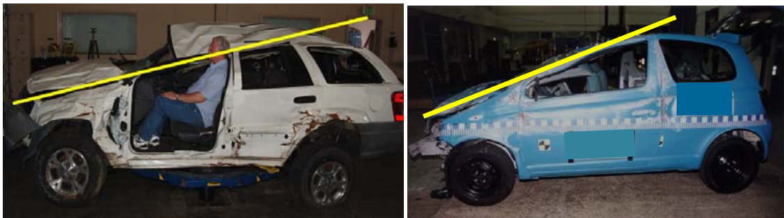
Figure 3: Note deformation line of A-pillar approximately matches yellow line shown. The line indicates how the vehicle has pitched forward during rollover as a result of the engine mass.
