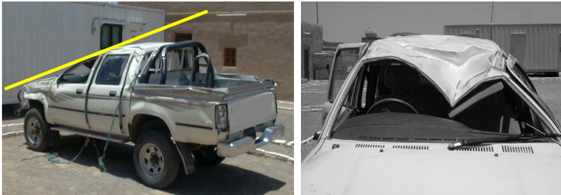
Figure 2: Vehicle reinforced with internal roll bar at B-pillar and external roll bar behind C-pillar. Note buckle of front windshield header rail intruding into occupant compartment.
