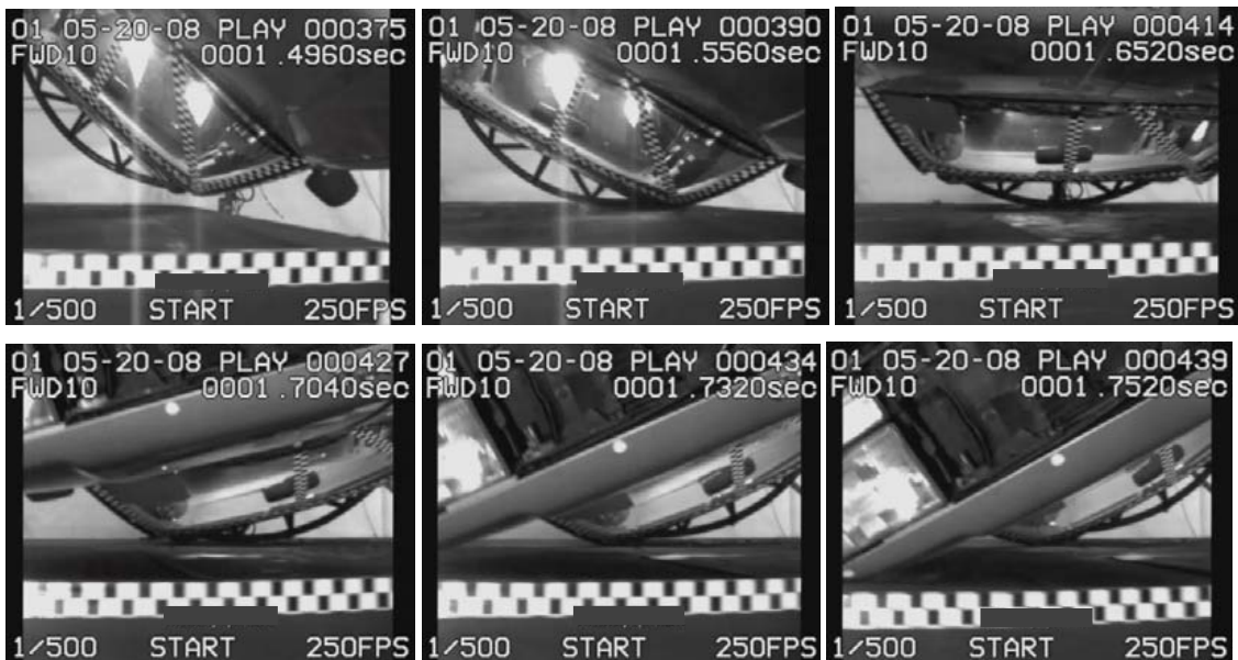
Figure 12: ATD interaction with (1993) low roof strength vehicle's (SWR 2.3) roof and floor during near side and far side touch down. ATD's head is circled.
