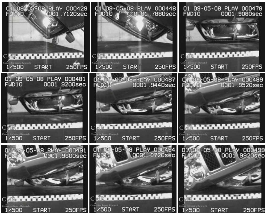
Figure 9: ATD interaction with low roof strength vehicle's (SWR 2.2) roof and floor during near side and far side touch down.
