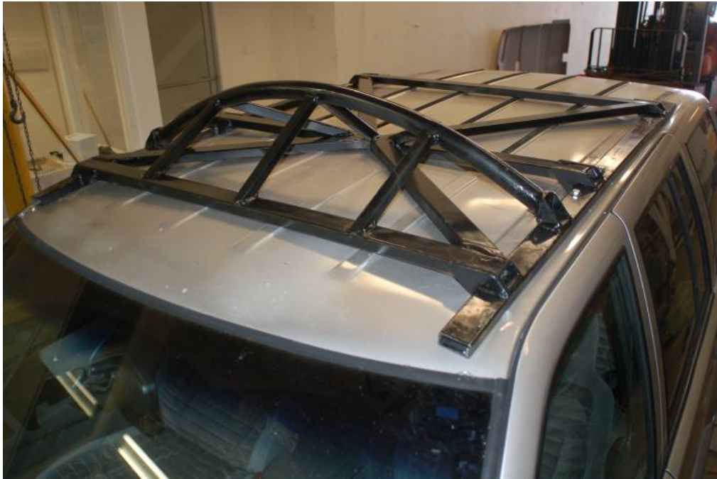
Figure 11: Prototype HALO™ fitted to roof of low strength (1993) vehicle.
