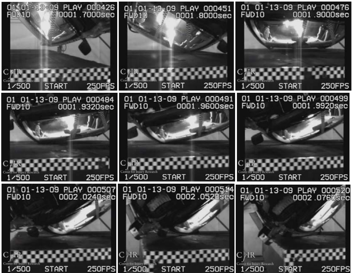
Figure 10: ATD interaction with high roof strength vehicle's (SWR 4.6) roof and floor during near side and far side touch down.
